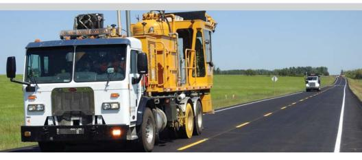
Paint represents the standard in road marking material. Paint application processes have evolved from a paint brush and can to large high speed trucks with laser or video guidance, fully instrumented to monitor all aspects of application with all data being uploaded into data warehouses. Precise accurate lines on any roadway can be achieved quickly and economically.
